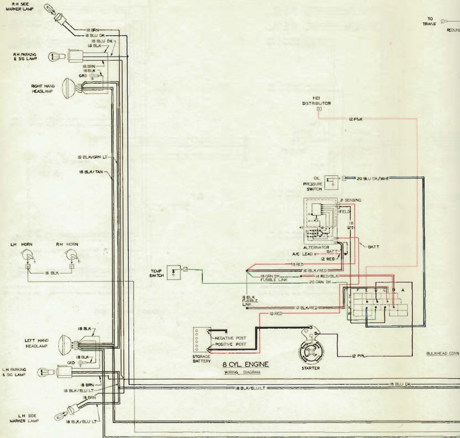
Fig. 8-24 F Series Wiring Schematics
